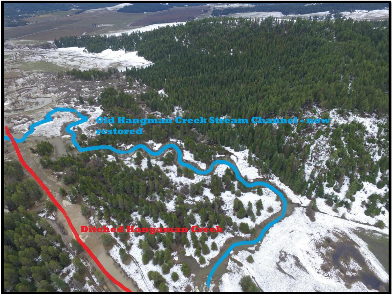
Figure 9. Restoration of Hangman Creek on the Coeur d'Alene Reservation. The ditched portion of the creek has been filled and the creek allowed to fill its historic channel on the flood plain.
